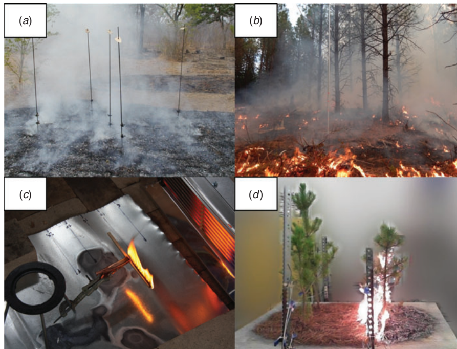
Fig. 1. Examples of highly instrumented outdoor ( a, b ) and indoor combustion laboratory experiments ( c, d ). ( a ) Experiment conducted to measure fire behaviour in a southern African savannah in 2001 (described in Smith et al. 2005); ( b ) Thermal radiometer towers deployed during mastication fires in 2014 (equipment description described in Kremens et al. 2012); ( c ) example ignition experiment following methods described by Finney et al. (2013); and ( d ) lodgepole pine ( Pinus contorta ) seedlings undergoing surface fires.
